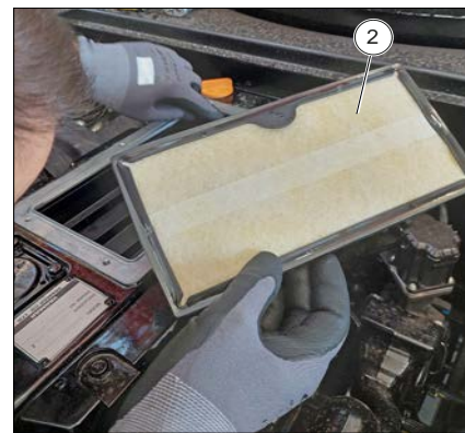
Figure 209: Replacement of the crankcase filter of the engine breather
