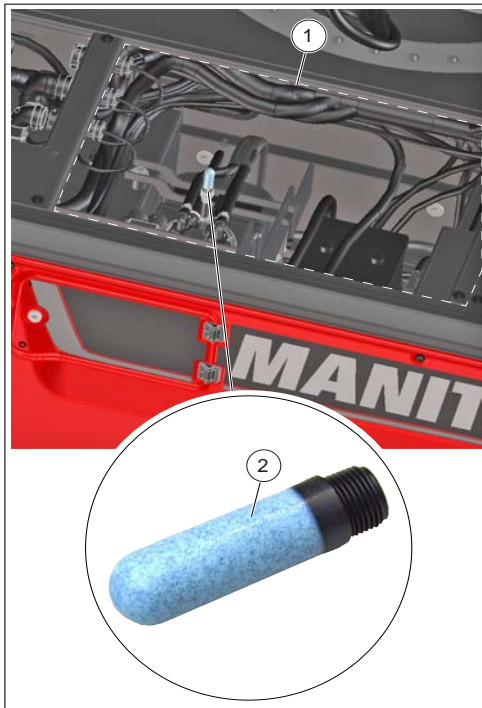
Figure 205: Replace the "DEF" tank breather
